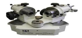
Computerized Double Flank Gear Roll Tester (Model: DO 125 K PC): **Procured and installed**
